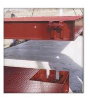
The OTR scale has an overlapping and interlocking joint design between panels which provides a significantly stronger joint than other models that use bolts to attach the panels together, which often shear after years of stress.
