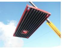
The quality of the OTR construction is the best in class. The manhole cover (on a pittype, concrete deck installation) is constructed from  $\frac{1}{2}$ " thick deck plate and uses 1" x 2" flat bar for the cover's support – most other manufacturers use  $\frac{1}{2}$ " plate with  $\frac{3}{8}$ " flat bar as support. Their concrete deck loadcell cover plate stiffeners are 1" flat bar welded
